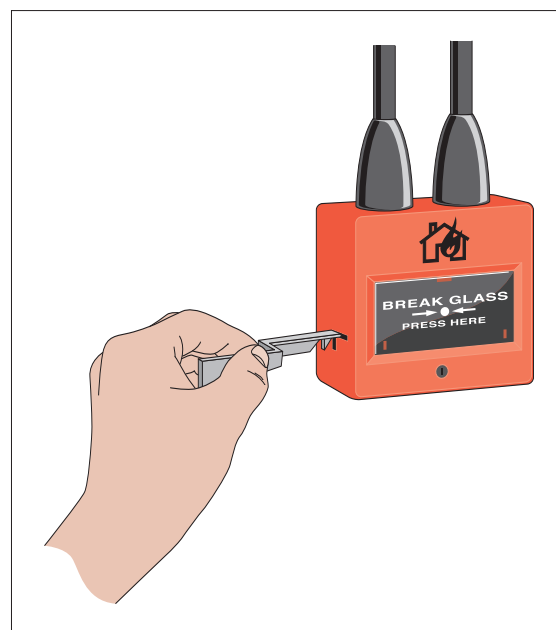
Figure 18: Using a test key
